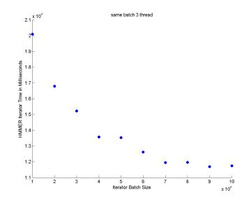
This graph was the best performance graph because it took much less time to process the data. With a thread size of 3 and a batch size of 100,000, we were able to process the data in about 12 seconds. The graph shows an exponential decrease that levels off when we increase the batch size.
