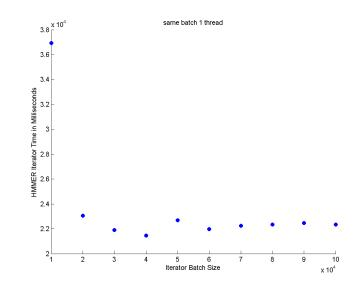
This is our worst performance graph. It uses only a single thread for the iterator. The time it takes for the iterator appears to be independent of the batchsize of a single thread.
